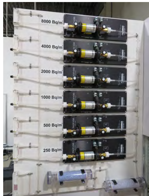
Source Panel made with several RN-1025 sources in parallel to provide an array of radon concentration for your chamber.
